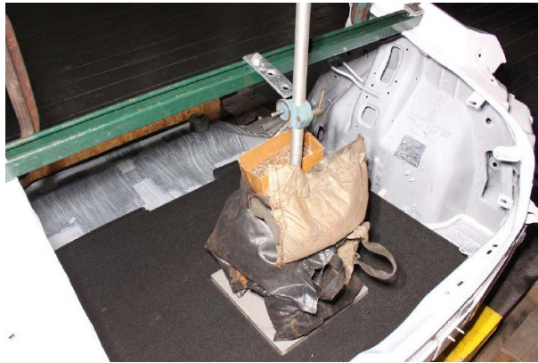
Figure 1: Load Application Using a Test Buck
