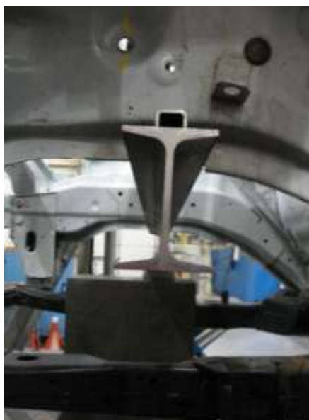
Figure 4: I-beam Located on the Front Wheel Wells
