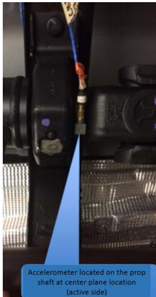
Figure 1: Active Side Accelerometer Location
