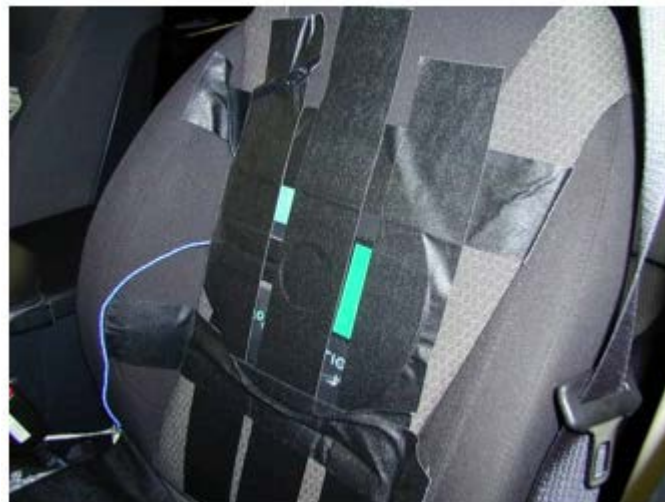
Figure 4: Seat Back Accelerometer Fixture
