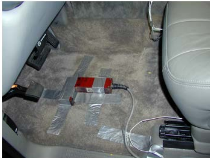
Figure 3: Floor/Feet Accelerometer Fixture
