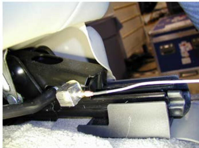
Figure 2: Seat Track Accelerometer
