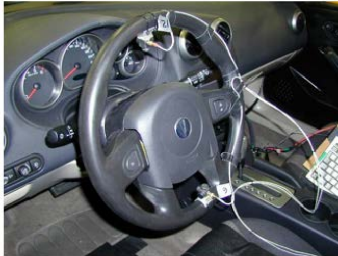
Figure 1: Steering Wheel Accelerometers
