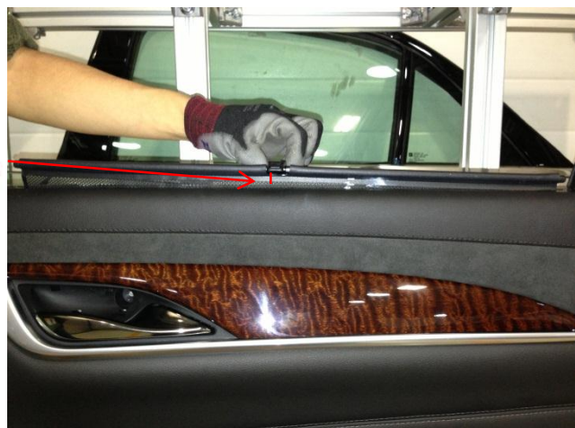
Figure 3: Measurement of Bottom Tension Force F3
