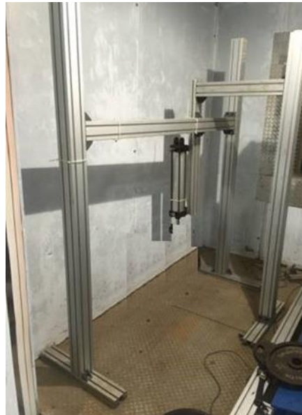
Figure 1: H-Frame Fixture Example
