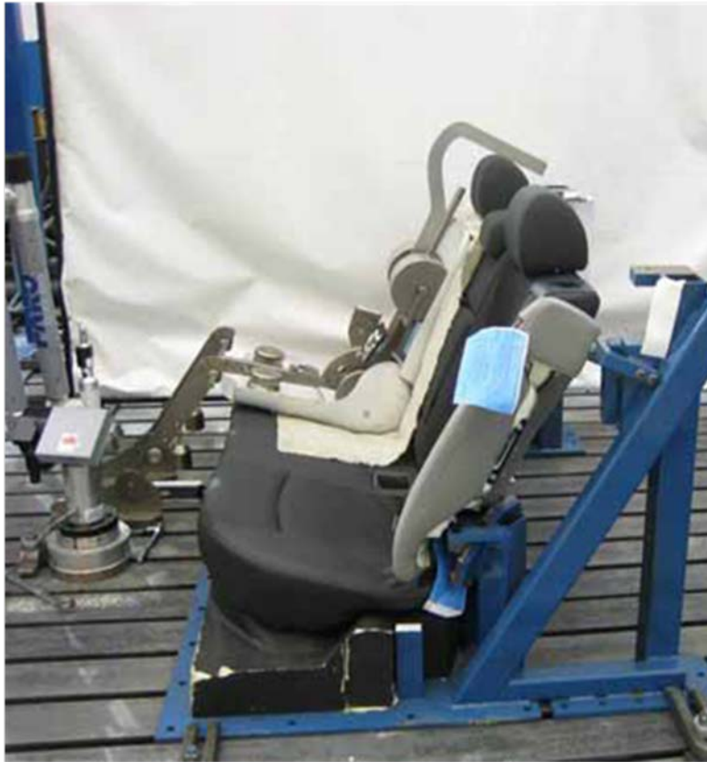
Figure 1: H-Point and Height Measurements
