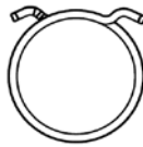
Figure 4: Clamp Type D, Normally Closed, Low Profile (Space Saver) (see Figure A4 for specifications)
