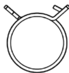
Figure 1: Clamp Type A, Normally Closed, Regular Profile (see Figure A1 for specifications)
