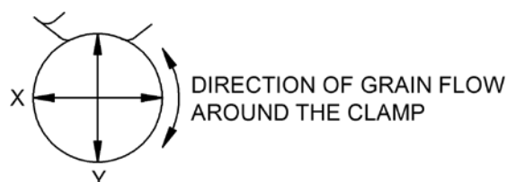
Figure 6: Clamp Shape and X-Y Directions of Hose Clamps
