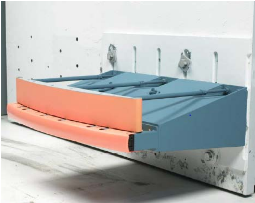
Figure 1: RCAR Barrier Test Device
