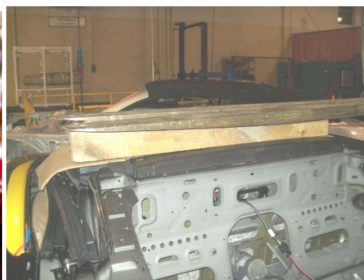
Figure 7: Obstruction across the Leading Edge of the Downstack
