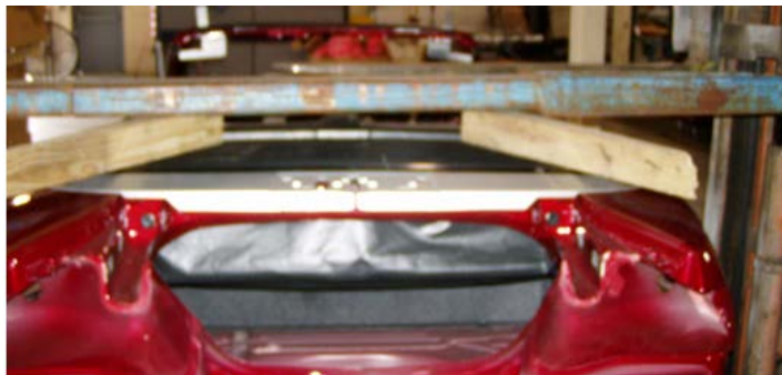
Figure 6: Obstruction from the Stowed Position at 45 Degrees across the Downstack
