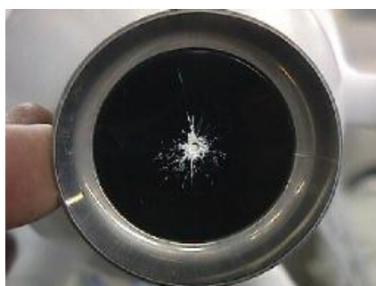
Figure 4: Cup Tested with Baseline Purge: Noticeable, but Not Excessive Residual Buildup
