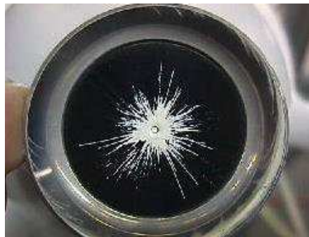
Figure 5: Cup Tested with Baseline Purge: Noticeable, but Not Excessive Residual Buildup
