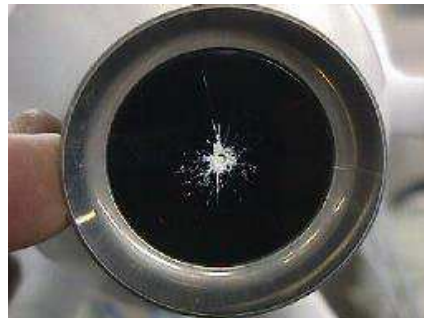
Figure 4: Cup Tested with Baseline Purge: Noticeable, but Not Excessive Residual Buildup
