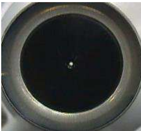
Figure 1: Cup Tested with Baseline Purge: No Residual Buildup (No Signal, Cleaning Cycle is too Severe)
