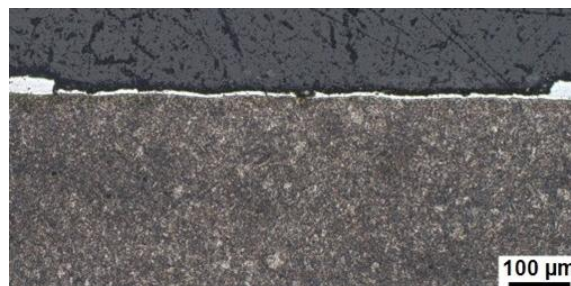
Figure 2: Example of Large Break-off Areas in AlSi Coated Hot Stamped Steel
