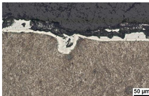
Figure 1: Example of Inversion in AlSi Coated Hot Stamped Steel
