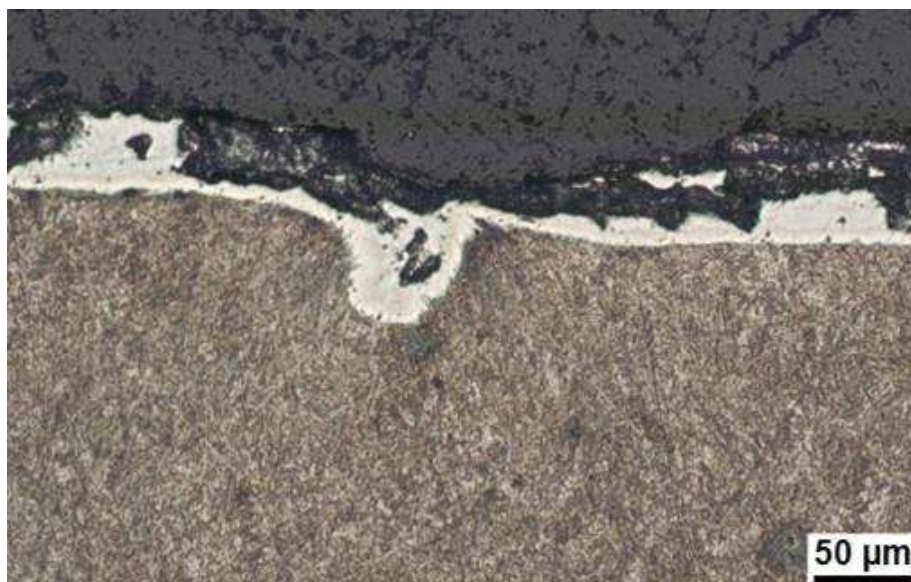
Figure 1: Example of Inversion in AISi Coated Hot Stamped Steel
