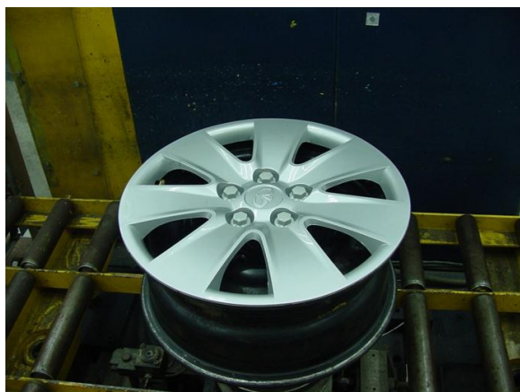
Figure 2: Cover installed to Wheel
