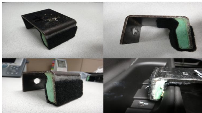
Figure 1: Pull Device with Epoxy Clay to Absorb Pull Cup Angle Variation
