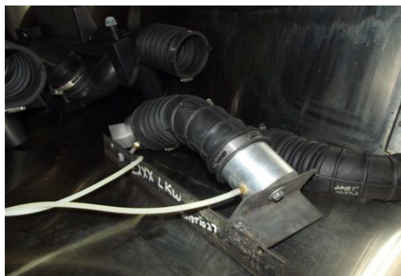
Figure 1: Vacuum Collapse Test Setup
