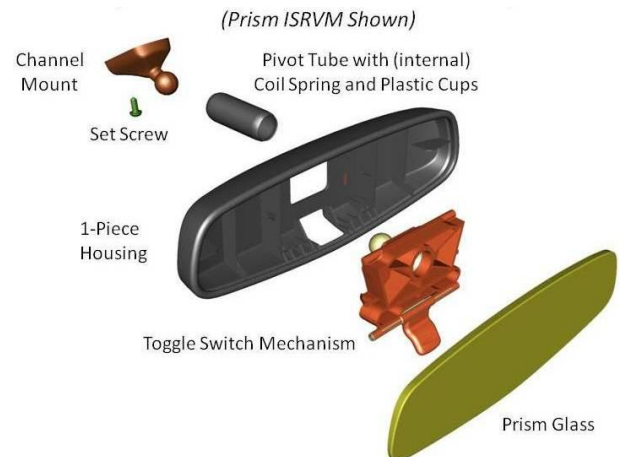
Figure 9: One-Piece Housing Construction
