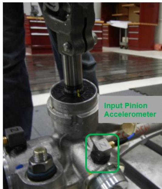
Figure 2: Column EPS Input Pinion Accelerometer Placement
