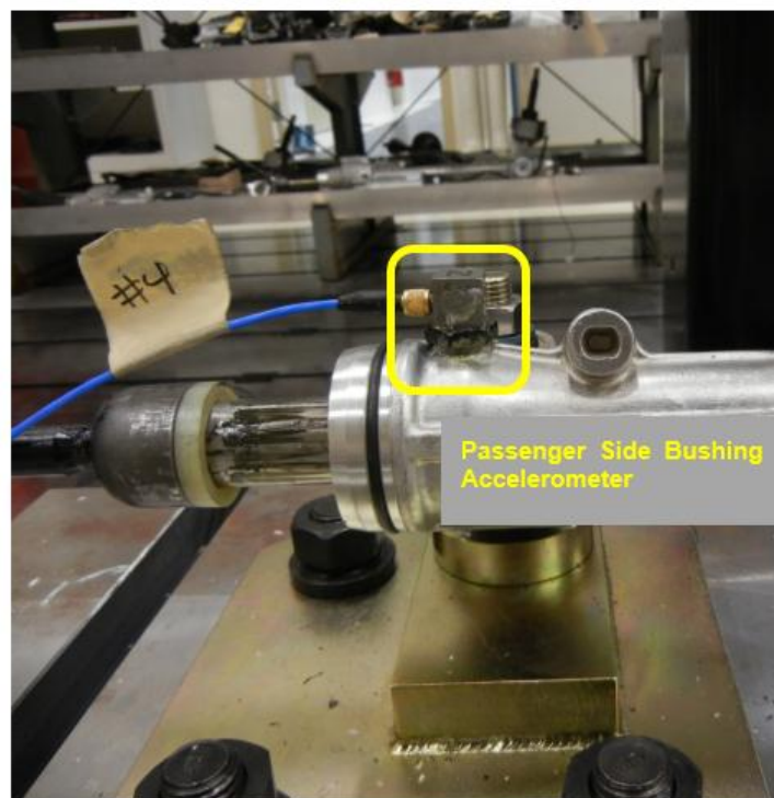
Figure 3: Column EPS Passenger Side Bushing Accelerometer Placement
