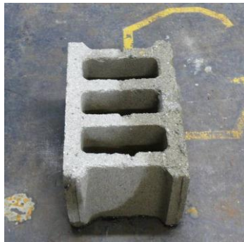
Figure 2: Concrete Building Block, 16 kg \pm 4 kg
