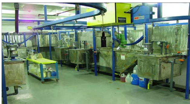
Figure 1: Example of Pretreatment Laboratory Line used for Panel Preparation
