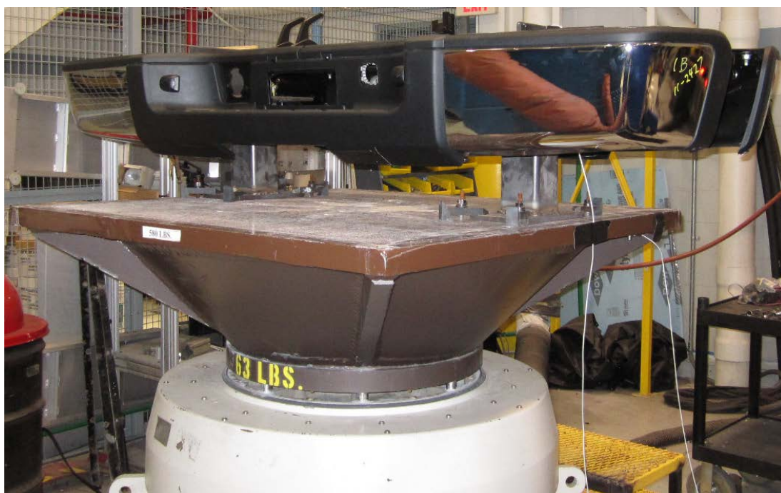
Figure 1: Bumper on Electro Dynamic Vertical Shaker Table
