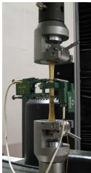
Figure 2: Tensile Specimen with an Axial and Transverse Extensometer Mounted
