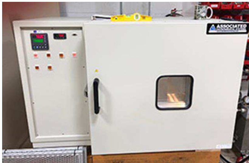
Figure 4: Temperature-Humidity Controlled Chamber
