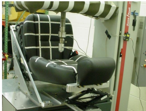
Figure 6: Seat Back Fixed, Indentation Normal to Torso Line Notice the Head Restraint Bars are Supported
