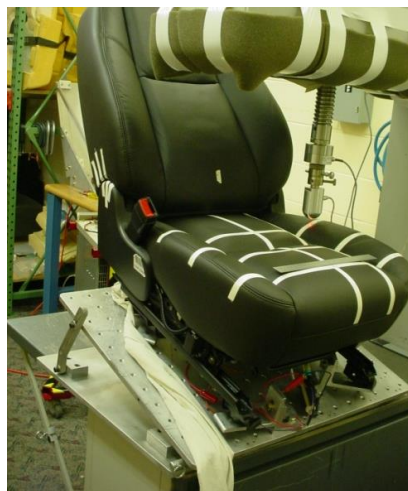
Figure 5: Seat Cushion Fixed, Indentation Normal to Thigh Line
