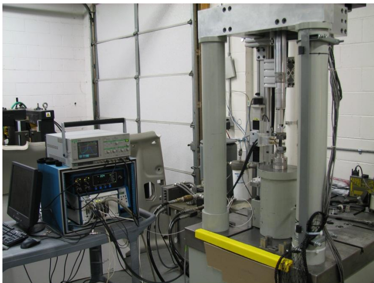
Figure 2: Tensile Testing Machine for Straining Rates between 1/s and 100/s
