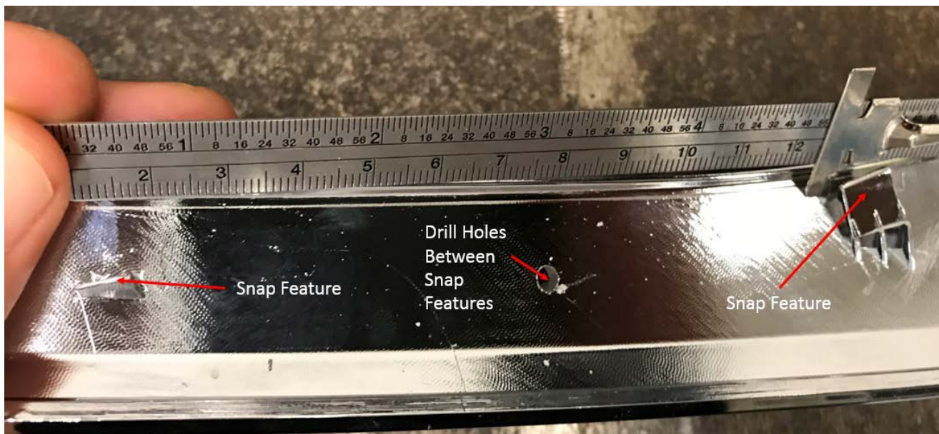
Figure 4: Hole Locations on A-side Part
