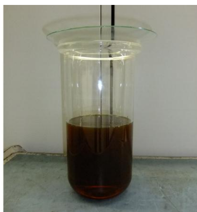
Figure 1: Example of Breaker With 50% Engine Oil
