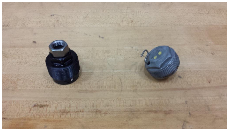
Figure 2: Mando Assembly with Retaining Nut (left), Nexteer Assembly with Grenade Pin (right)
