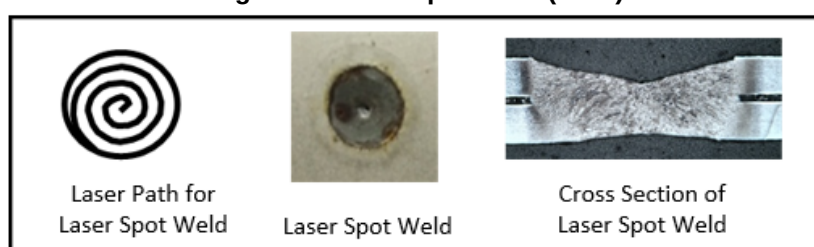
Figure 2: Laser Spot Weld (LSW)
