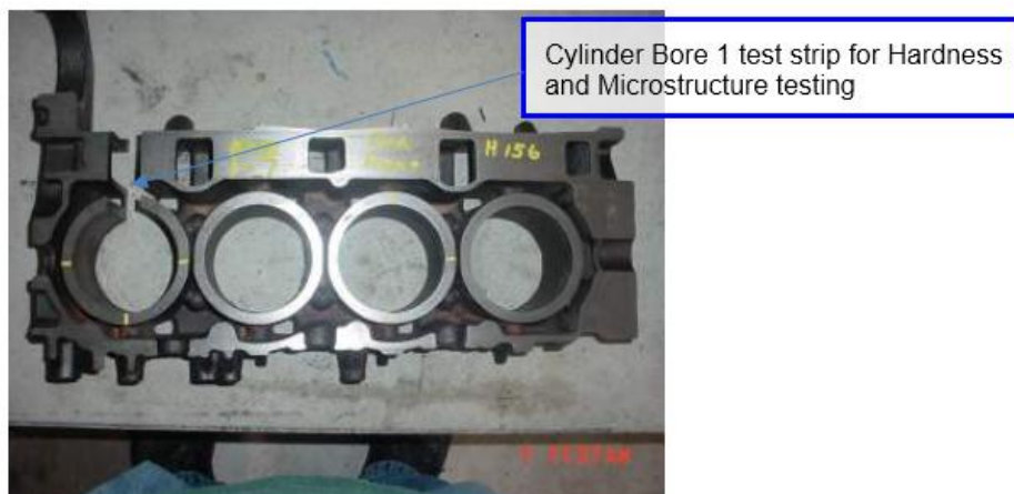
Figure 2: Example of Head Deck Sectioned for Microstructure and Bore Wall Hardness Check on Bore No. 1
