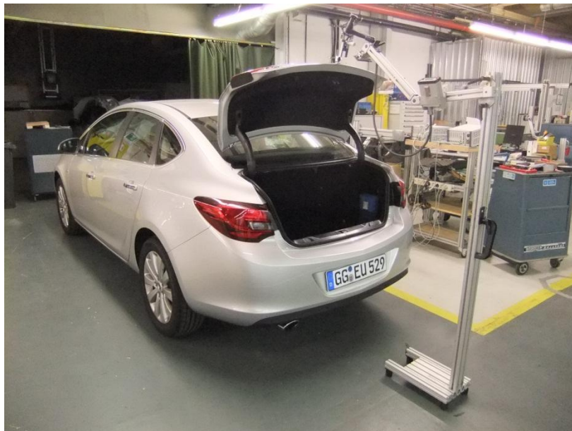
Figure 1: Test Set up “Deck Lid Opening Velocity” measured 5° from the Static Full Open Position
