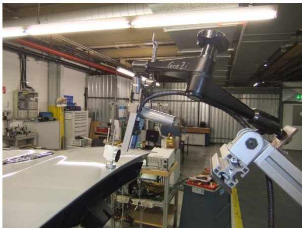
Figure 2: Test Set up “Deck Lid Opening Velocity”, Interrupter and sensor of the Velocity Meter aligned without contact while opening of the deck lid
