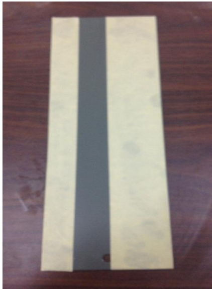
Figure 1: “Taped Test Panel” for Bead Masking and Location
