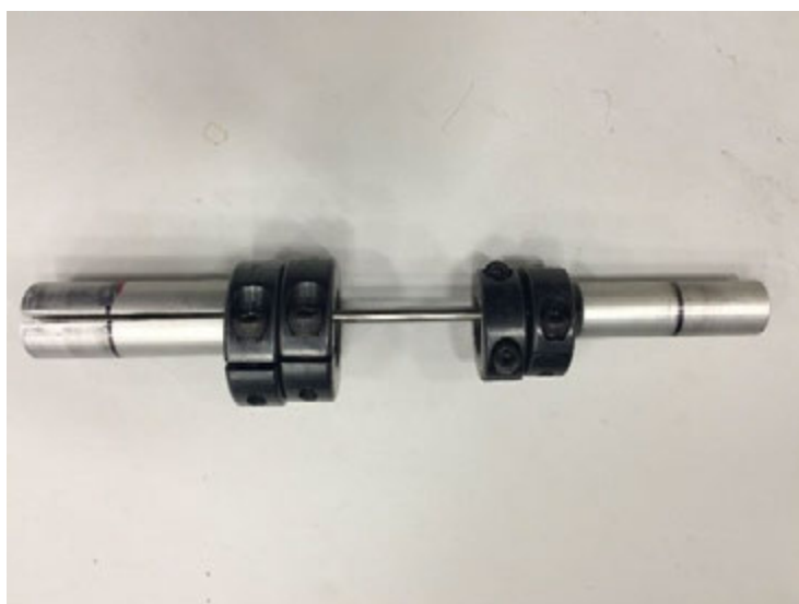
Figure 7: Torsion Spring with the Shaft Collars and Adaptors
