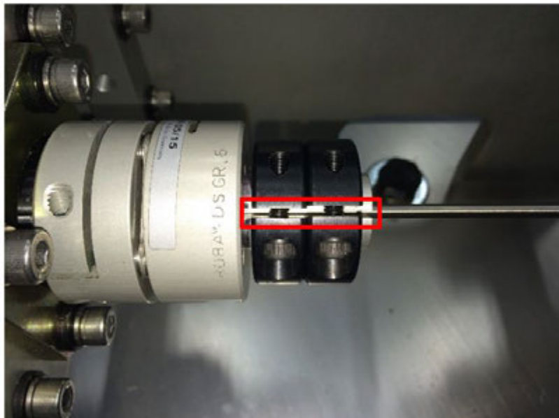
Figure 9: Aligning the Shaft Collar Slit to the Torsion Spring Adaptor Slit before Tightening
