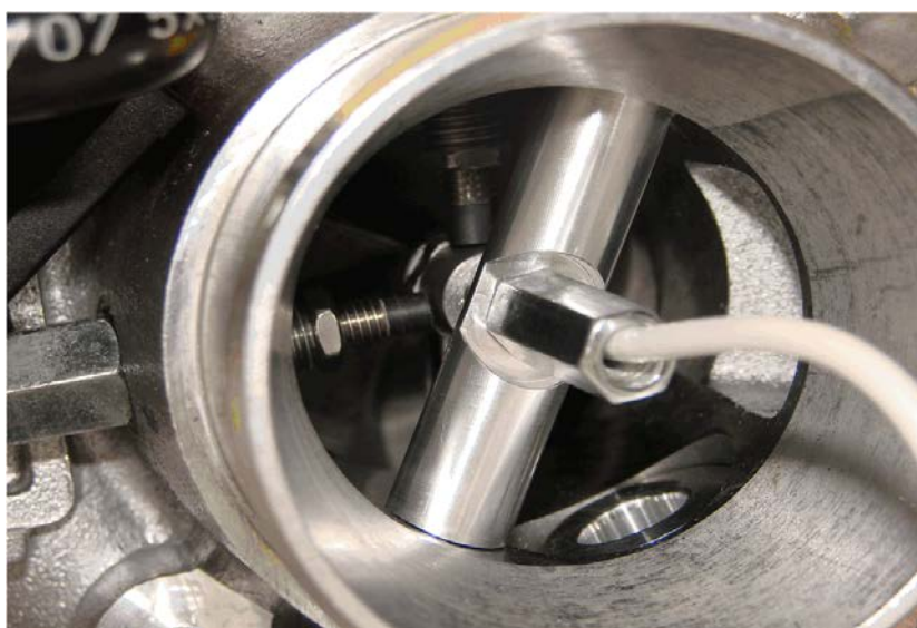
Figure 2: Turbocharger with Proximity Sensor
