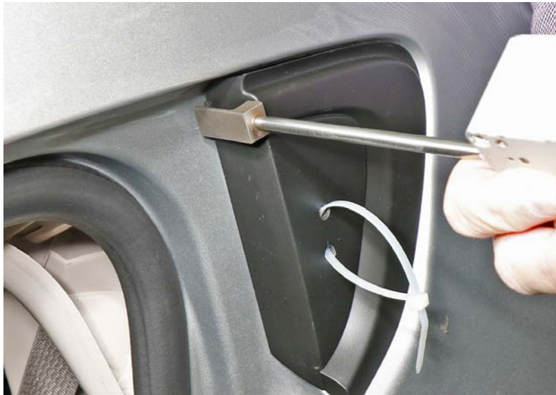
Figure 3: Pillar Applique Peel
