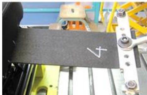
Figure 2: Clamping Device used to pull the Coupon with an Evenly Distributed Load
