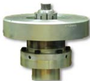
Figure 4: GMNA – Spindle Tooling with Collet
