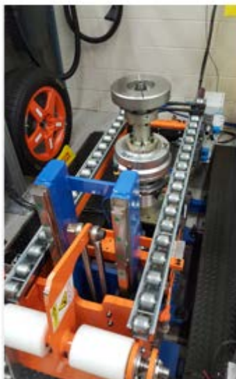
Figure 1: Tire Wheel System (TWS) Dynamic Balancer
