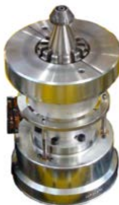
Figure 5: Assembly Plant Multi-Jaw Tooling
