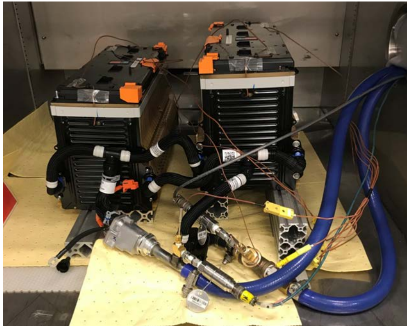
Figure 4: Cooling System Setup Example, Inside Chamber
