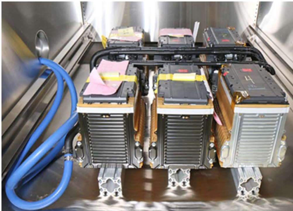
Figure 1: Environmental Chamber Test Set-up Example using Battery Electric Vehicle (BEV) Sections
