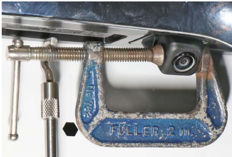
Figure 7: Camera with Clamp Installed
