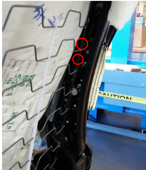
Figure 1: Image of Inflator Attachment to Seat Back Frame Side Member
