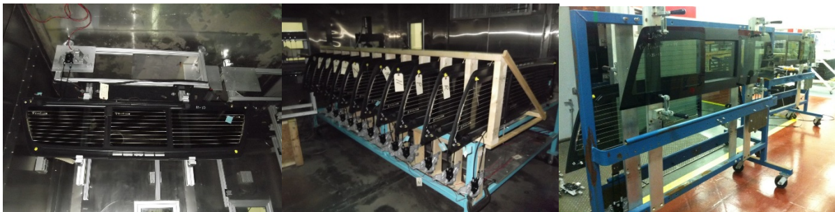
Figure 2: Examples of Test Fixture/Holding Fixture
