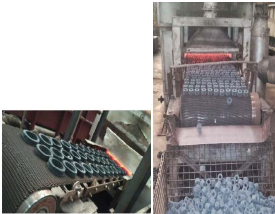
Figure 1: Example of Single Layer Loading Required for Heat Treatment of Powertrain Gears
