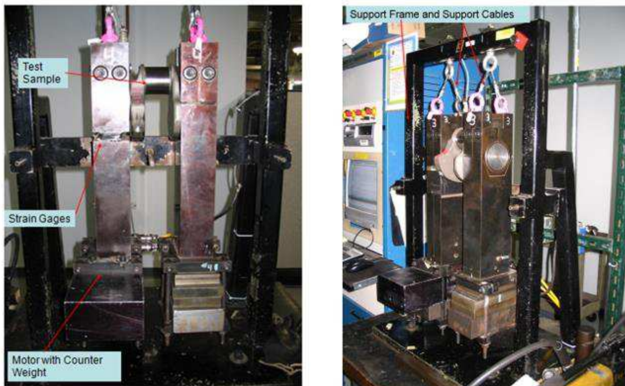
Figure 1: Example Tuning Fork Fixture Setup
