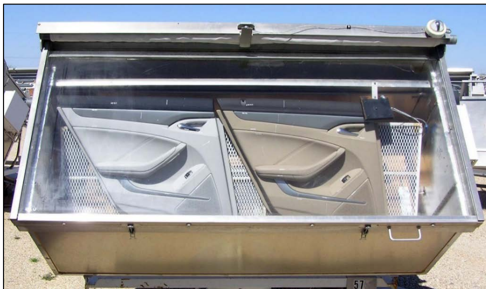
Figure 4: Code F2 Test Fixture with Door Trim
