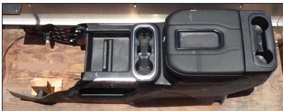
Figure 2: Code F2 Test Fixture with Floor Console Assembly
