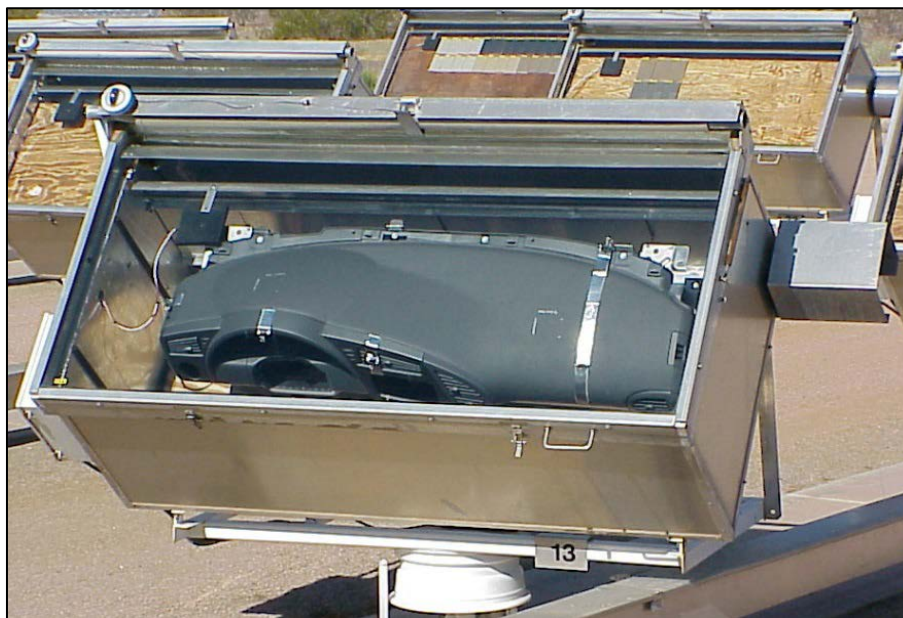
Figure 1: Code F2 Test Fixture with Instrument Panel Trim Assembly
