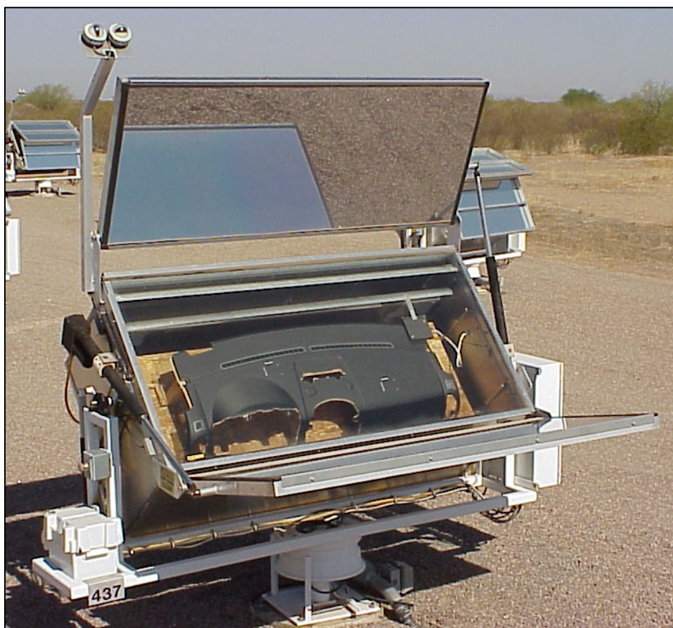
Figure 5: Code F3 Test Fixture with Instrument Panel Upper Trim
