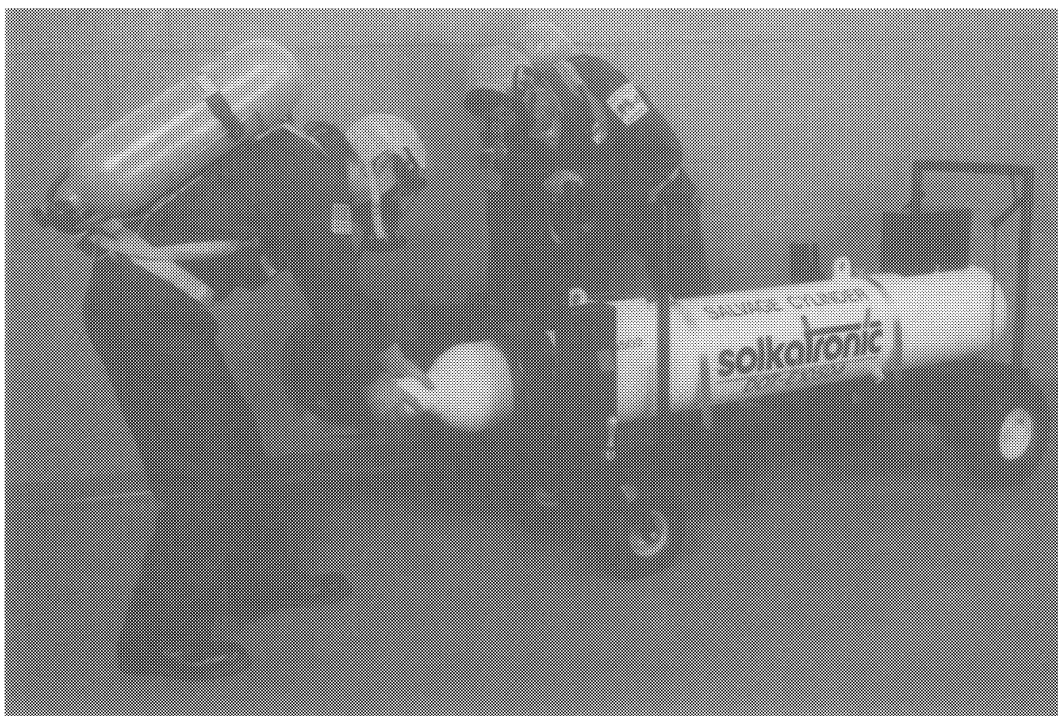
Fig. 2-2. Emergency response team trains for containment of a leaking cylinder using a cylinder containment vessel.
