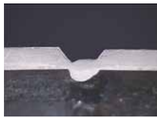
Excessive root reinforcement
