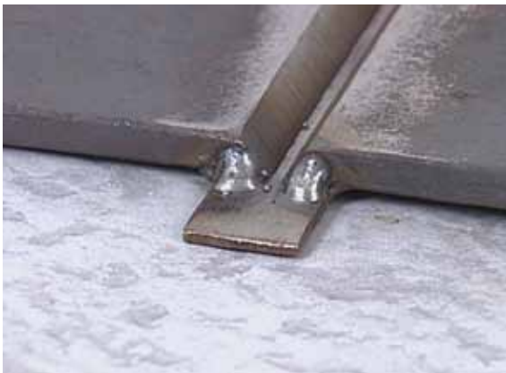
Proper joint fit-up.
