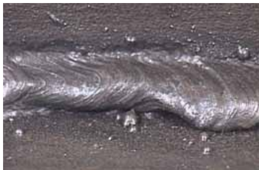
Overlap of a weld
