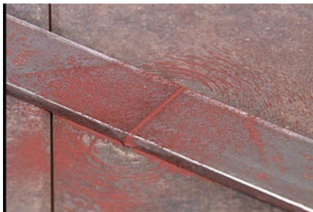
Magnetic Particle Testing
