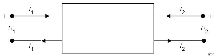
Figure 1 – Conventions concerning signs in electric circuits
