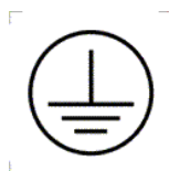
Figure 3 – Symbol for protective earth (protective ground)
